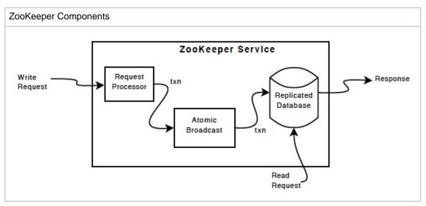
The replicated database is an in-memory database containing the entire data tree. Updates are logged to disk for recoverability, and writes are serialized to disk before they are applied to
