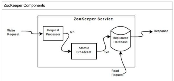
The replicated database is an in-memory database containing the entire data tree. Updates are logged to disk for recoverability, and writes are serialized to disk before they are applied to the in-memory database.
